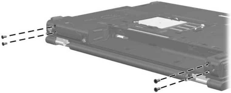
Removing the Display Assembly Screws
