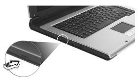
When the power is off, you can eject the drive tray by using the emergency eject hole.
