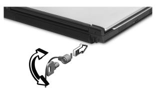
Wrap the computer security lock cable around an immovable object such as a table or handle of a locked drawer. Insert the lock into the notch and turn the key to secure the lock. Some keyless models are also available.
